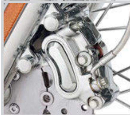
B. FRONT BRAKE CALIPER KIT – CHROME (SHOWN WITH CHROME CALIPER BOLT COVER KIT AND CALIPER INSERT)
