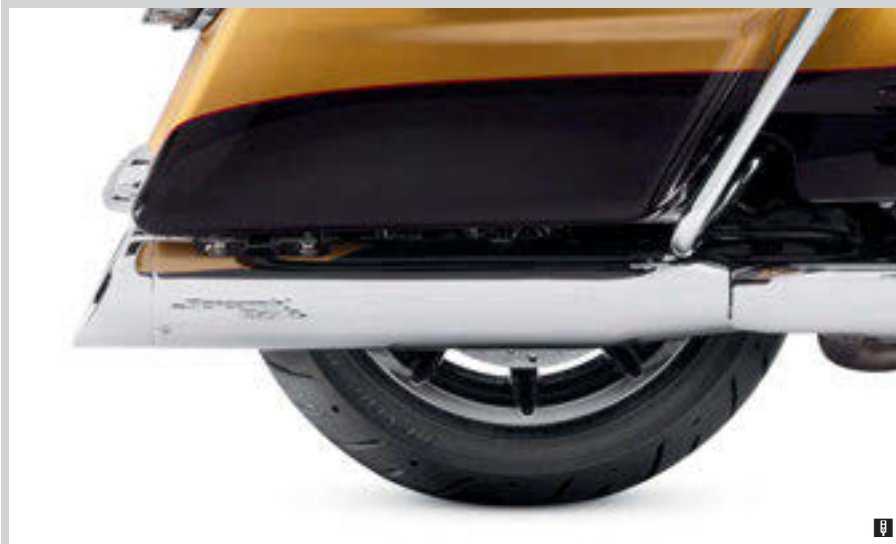
C. SCREAMIN' EAGLE STREET CANNON PERFORMANCE SLIP-ON MUFFLERS – 4.5" – CHROME (SHOWN WITH CHROME TWO-PIECE END CAPS)
