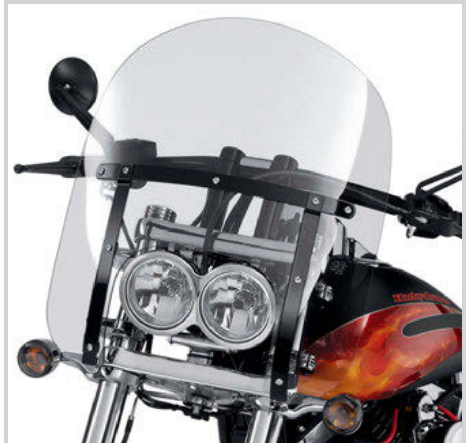
A. QUICK-RELEASE COMPACT WINDSHIELD – 15", GLOSS BLACK BRACES (SHOWN WITH TURN SIGNAL RELOCATION KIT)
