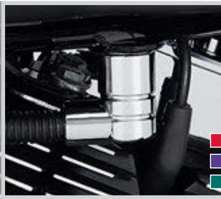
F. FUEL TANK FITTING COVER
