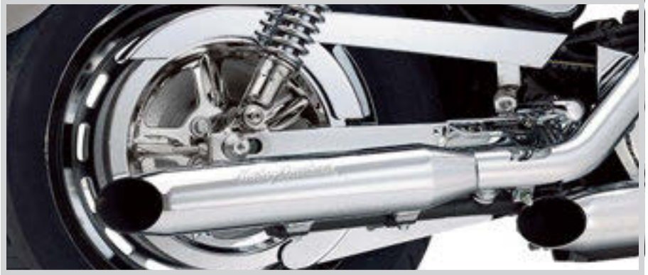
A. UPPER BELT GUARD – CHROME (SHOWN WITH CHROME LOWER BELT GUARD AND SWINGARM)
