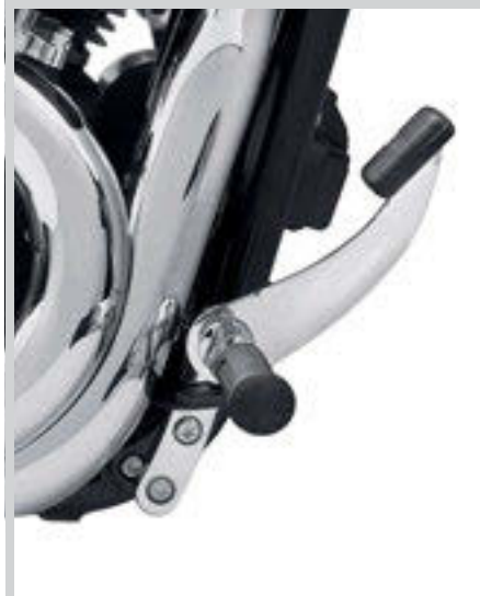
REDUCED REACH FORWARD CONTROLS
